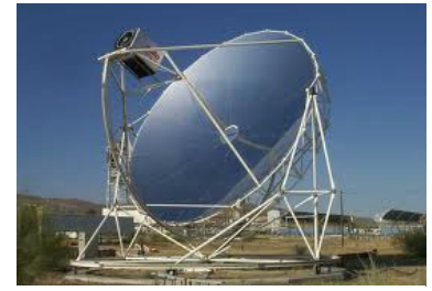
Stirling Engine mounted on a Solar Dish
