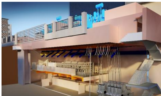
Underground GIS at 'Quest Mall'
