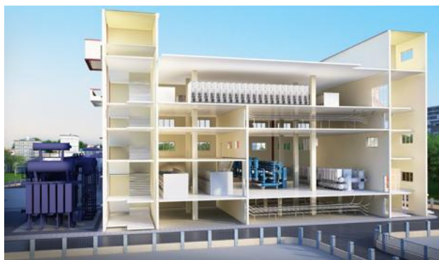
Integrated SS at New Cossipore with 220, 132 & 33 kV GIS
