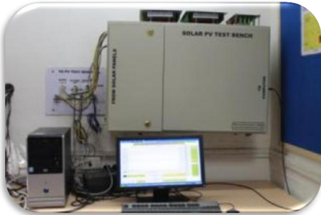
PV Test-bed for Testing Ten (10) Solar PV Modules Simultaneously
